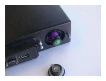
**5.** Use the battery compartment cover to push the battery into the compartment, aligning the tabs on the cover with the compartment slots. Twist the cover clockwise to lock the compartment.
